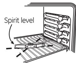
C The rear leveling legs must be adjusted prior to moving the range into position. They can be adjusted from the bottom at the back of the range.
