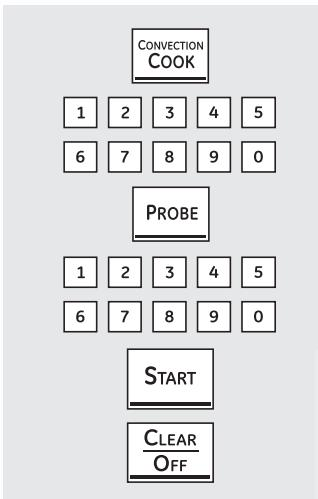
To change the oven temperature during the Convection Roast cycle, touch the **CONVECTION COOK** pad and then touch the number pads to set the new desired temperature.
