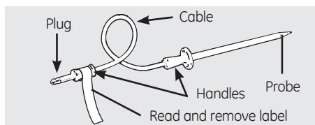
■ Never leave your probe inside the oven during a self-cleaning or broil cycle.
