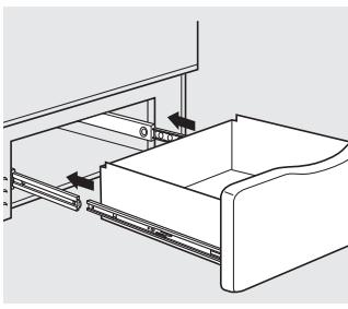
**2** Press the left rail release up and press the right rail release down, while pulling the drawer forward and free.
