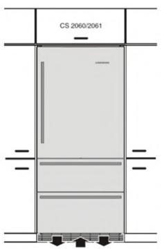
CS/CBS 20 appliances dont need any ventilation openings in the cabinet. The required airflow is directed through the toe kick area.
