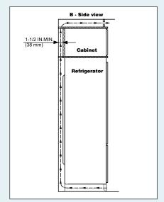
Do not restrict the air flow. The opening can either be directly over the appliance ①, above the cabinet and below the ceiling ② or through a vent installed in a soffit ③.
