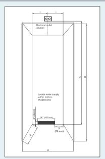
\*The given cabinet opening height dimension includes space for top air vent. If you choose to place the vent above the cabinet or in a soffit, you will need to adjust the height dimensions accordingly. Please refer to Ventilation Requirements. The appliance can be integrated into the kitchen units. To adapt the appliance to the height of the row of kitchen units, a suitable top cupboard can be fitted above the appliance.
