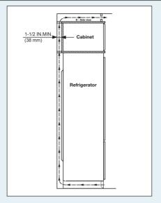
This type of cabinet must be carefully constructed using the correct dimensions and it must provide suitable ventilation to ensure proper appliance operation.
