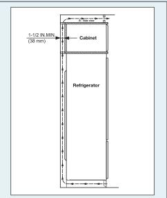
This type of cabinet must be carefully constructed using the correct dimensions and it must provide suitable ventilation to ensure proper appliance operation.
