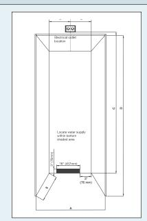
\*The given cabinet opening height dimension includes space for top air vent. If you choose to place the vent above the cabinet or in a soffit, you will need to adjust the height dimensions accordingly. Please refer to Ventilation The appliance can be integrated into the kitchen units. To adapt the appliance to the height of the row of kitchen units, a suitable top cupboard can be fitted above the appliance.
