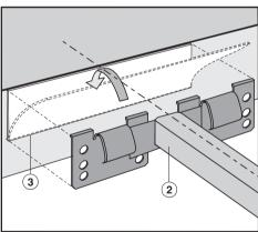
■ Position and attach the spring clips
