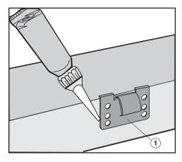
■ Coat the side and lower edges of the spring clips between ① and ② with silicone.
