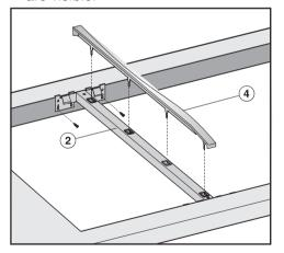
■ Insert the sealing strip ④ into the holes in the support bar ②.
