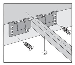
■ Place the supplied spring clips ① and the support bars ② at the marked positions as shown above, by laying them on the upper edge of the cut-out and then securing them with the ¹/₀" x 1" (3.5 x 25 mm) screws (supplied).
