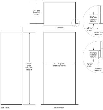
NOTE:  $3^{1/2^*}$  (89) finished returns will be visible and should be finished to match cabinetry Shaded line represents profile of unit.
