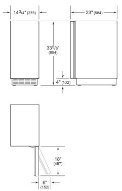
**IMPORTANT NOTE:** Overall dimensions do not include panels or handles. Dimensions will vary with panel thickness.
