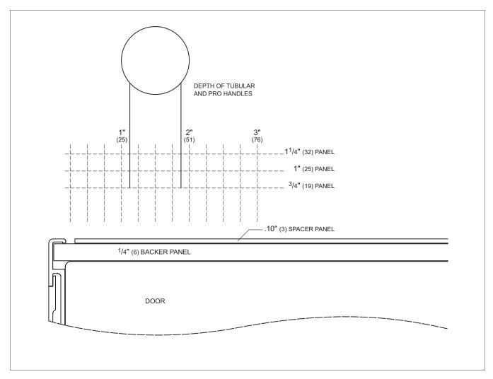
Overlay and flush inset panel thickness
