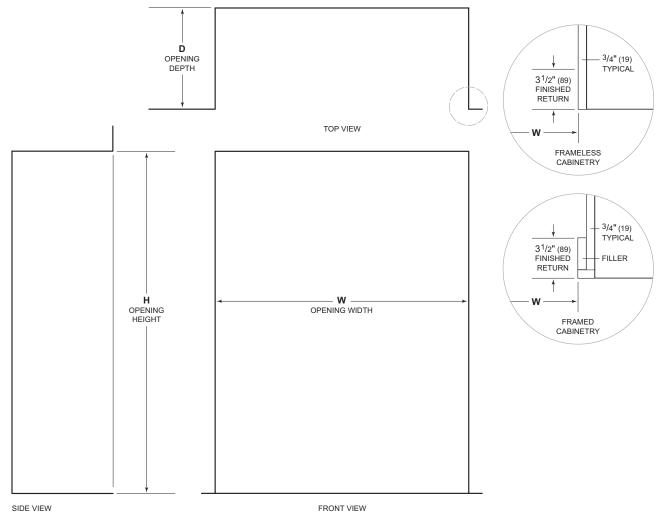
NOTE: 3<sup>1</sup>/2" (89) finished returns will be visible and should be finished to match cabinetry.
