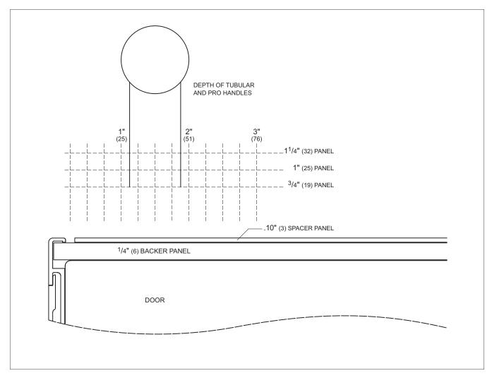
Overlay and flush inset panel thickness
