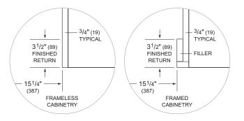
The depth of the unit is 23" (584). Allow for panel thickness when planning the finished opening depth. A minimum  $3\frac{1}{2}$ " (89) finished return is required on all sides of the opening. Framed cabinets require additional finished filler material behind the face frame for a proper installation. Refer to the illustration above.
