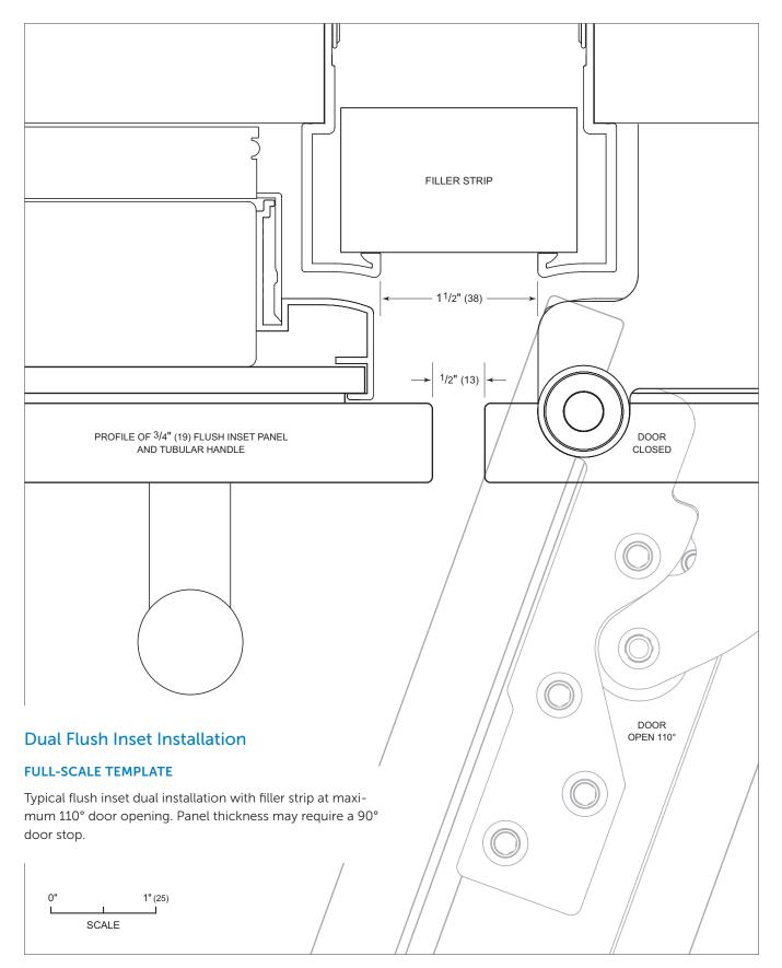
Dual flush inset installation (top view)
