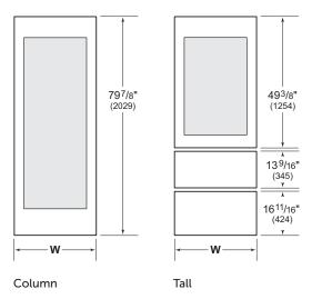
Typical panel dimensions are based on an 84" (2134) finished height, 4" (102) toe kick, and ¼" (3) reveals. Panel dimensions must be adjusted accordingly for all other installations. Refer to the illustration for panel height and the chart below for panel width.
