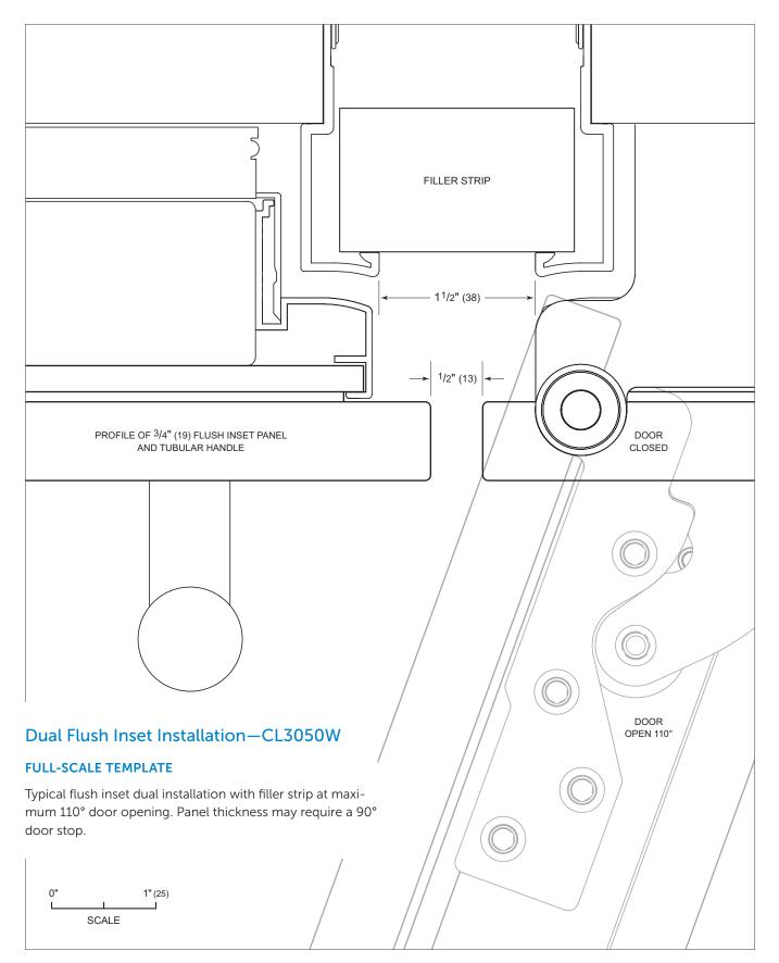
Dual flush inset installation (top view)
