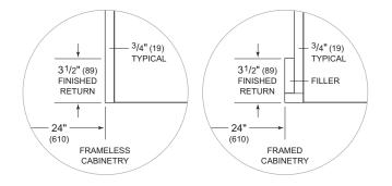
The depth of each model is  $23\frac{1}{8}$ " (587). Allow for panel thickness when planning the finished opening depth. A minimum  $3\frac{1}{2}$ " (89) finished return is required on all sides of the opening. Framed cabinets require additional finished filler material behind the face frame for a proper installation. Refer to the illustration.
