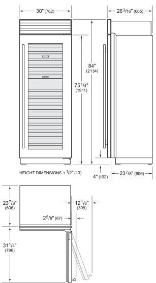
**IMPORTANT NOTE:** Overall dimensions are based on the stainless steel model. For flush inset applications, add <sup>1</sup>/2" (13) to door clearance dimensions.
