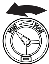
Counterclockwise to reduce foaming
