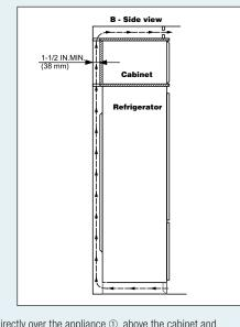
Do not restrict the air flow. The opening can either be directly over the appliance ①, above the cabinet and below the ceiling (2) or through a vent installed in a soffit (3).
