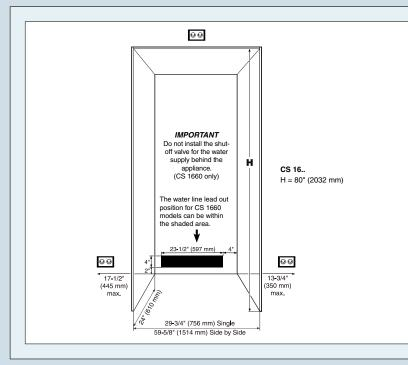
The appliance can be used freestanding or semi built-in. If semi built-in, consider the cabinet opening dimensions.
