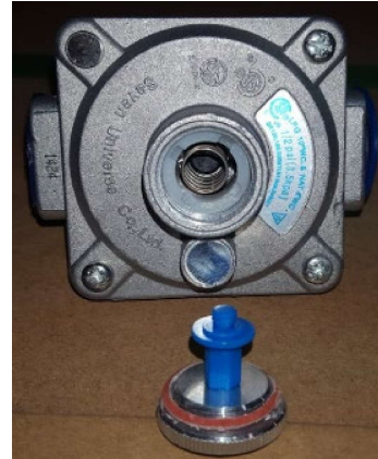
Image of the regulating pole set to LP.
