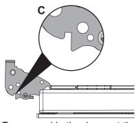
To reassemble the door, put the hinges in the relevant slots in the oven, making sure that grooved sections C are resting completely at the bottom of the slots. Lower the door and once it is in place remove the pins from the holes in the hinges.
