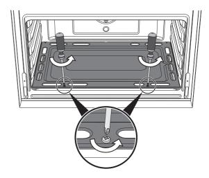
3) Lift the oven floor and slide it out.
