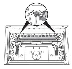
3) Remove the burner by sliding it from its place and reposition it as shown in the picture. (Make sure not to damage the thermocouples and the spark electrode).
