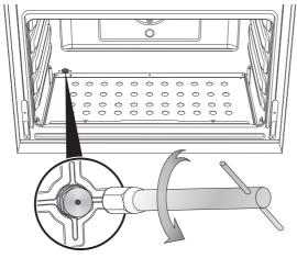
6) Using a 7mm socket wrench replace the nozzle, installing the one that is appropriate for the type of gas to be used. Refer to the gas charts at point 5.
