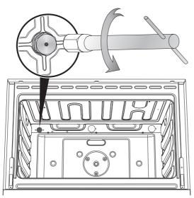
4) Using a 13mm socket wrench replace the nozzle, installing the one that is appropriate for the type of gas to be used. Refer to the gas charts at point 5.
