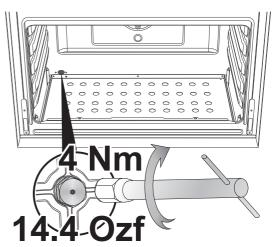
**7) WARNING**: The tightening torque of the nozzle must be equal to 4 Nm.
