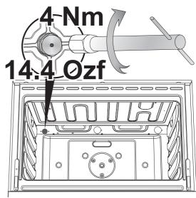
5) WARNING: The tightening torque of the nozzle must be equal to 4 Nm - 14.4 Ozf.
