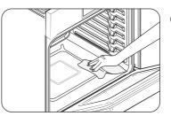
Clean the oven's interior. There will be a significant amount of water remaining on the bottom of the oven after a steam-cleaning cycle. Remove the residual water with a sponge or soft dry cloth.
