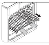
With the Gliding rack in the Closed position and the oven off and cool, grasp the rack and frame and pull both forward to remove.
