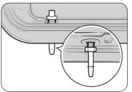
2. Insert the steam nozzle into the hole on the right-rear side of the metal pan, and then tighten the provided nut.
