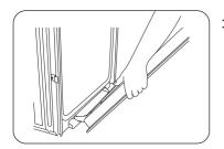
Hold the door at a 45 ° angle, and then 3. align the door hinges with the slots in the lower front of the oven cavity. Slowly insert the door, making sure you maintain the 45 ° angle. You will know the door is engaged in the slot when vou feel a slight drop.
