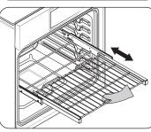
When using the Gliding rack in the oven, be sure to pull on the handle of the rack only to slide it in and out. If you grasp the frame while using the rack, the entire Gliding rack will be removed. Make sure you use oven gloves when handling the Gliding rack during cooking.
