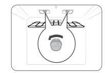
**3.** Turn the bulb cap counterclockwise to remove.
