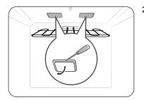
2. While holding the glass cover with one hand, insert a flat-sharp tool such as a table knife between the glass and the frame to remove the glass cover.
