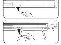
Shake the graphite lubricant before opening it. Starting with the left (front and back) slide mechanism of the rack, place four (4) small drops of lubricant on the two (2) bottom tracks of the slide close to the bearing carriers
