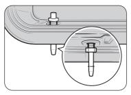
Insert the steam nozzle to the hole on the right-rear side of the metal pan, and then tighten the provided nut.
