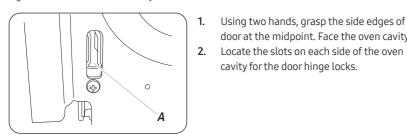
A. Slot in the oven cavity for the door hinge lock
