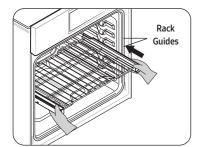
With the Gliding rack in the Closed position and the oven off, carefully insert the Gliding Rack between the guides until the rack reaches the back.
