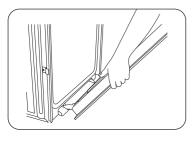
Hold the door at a 45 ° angle, and then align the door hinges with the slots in the lower front of the oven cavity. Slowly insert the door, making sure you maintain the 45° angle. You will know the door is engaged in the slot when you feel a slight drop.
