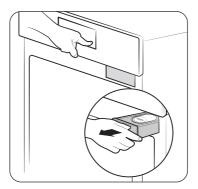
Locate the water reservoir. The water reservoir is on the right side of the oven, just above the oven opening. Touch Open/Close Reservoir on the control panel to eject the water reservoir.
