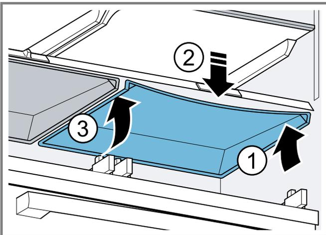
If the fruit and vegetable container cover is still bent, move the humidity regulator to and fro until the fruit and vegetable container cover clips into place.
