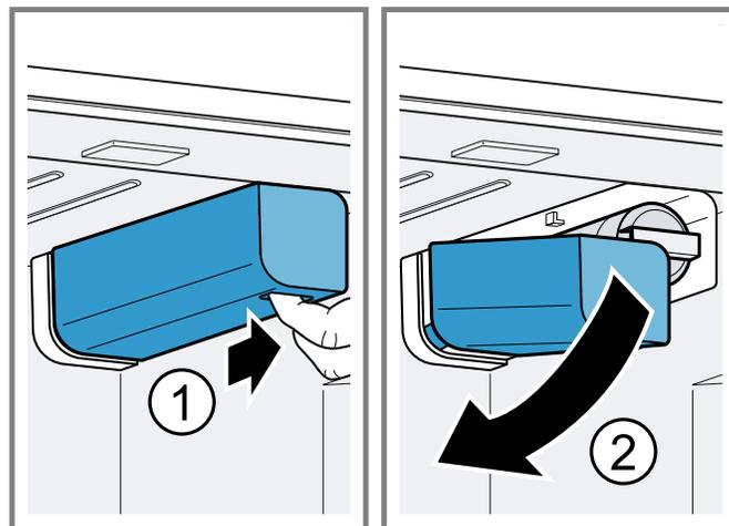
2. Pull the water filter down to the left ①, turn it counterclockwise by 90° ② and remove it ③.
