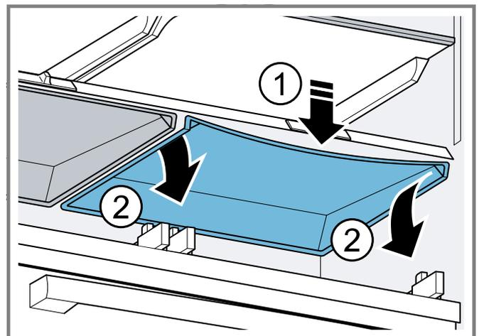
3. Pull out the fruit and vegetable container cover at the rear ① and remove it ②.
