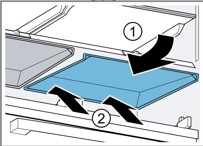
2. Clip in one side of the fruit and vegetable container cover at the front ①, then bend it downward slightly at the middle ②, and then clip in the other side at the front ③.
