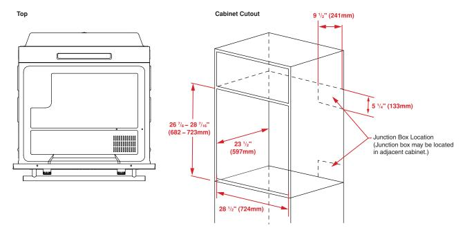
If installing in lower cabinet, leave 4" (102mm) min clearance below.
