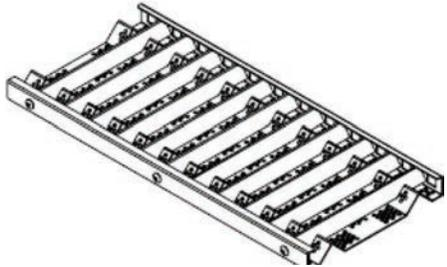
Years of design technology is placed into this “one of a kind” vaporizer with Stainless Steel pyramid style flavor bars and specially designed evaporation plates. This flame tamer pump’s even heat onto the food at the same time as vaporizing overflow juices that create added flavor in the food.
