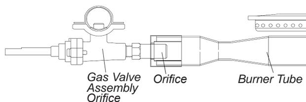
Please Note that the air mixture for LP gas and NG is different. Your gas BBQ will come preset for your gas type. If you find that you are not getting the best flame you can adjust the air shutter and the O2 mix with gas will change the flame. The flame coming from your burner is extremely important. If the flame is not correct you will be able to adjust the flame as described in the section below.
