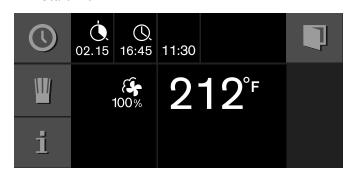
The appliance assumes a waiting mode. The operating mode, the temperature, the cooking time and the end of the cooking time appear in the display. The
