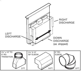
The system will operate most efficiently when the ductwork does not exceed 40 feet of equivalent duct. The chart above, shows equivalent feet of elbows and transitions. The number of feet of straight 31/4" x 10" or 6" duct plus the equivalent feet of elbows or transitions to be used should equal 40 feet or less.
