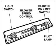
The **blower speed control** changes the running speed of the blower. It is infinitely adjustable from low to high speed.
