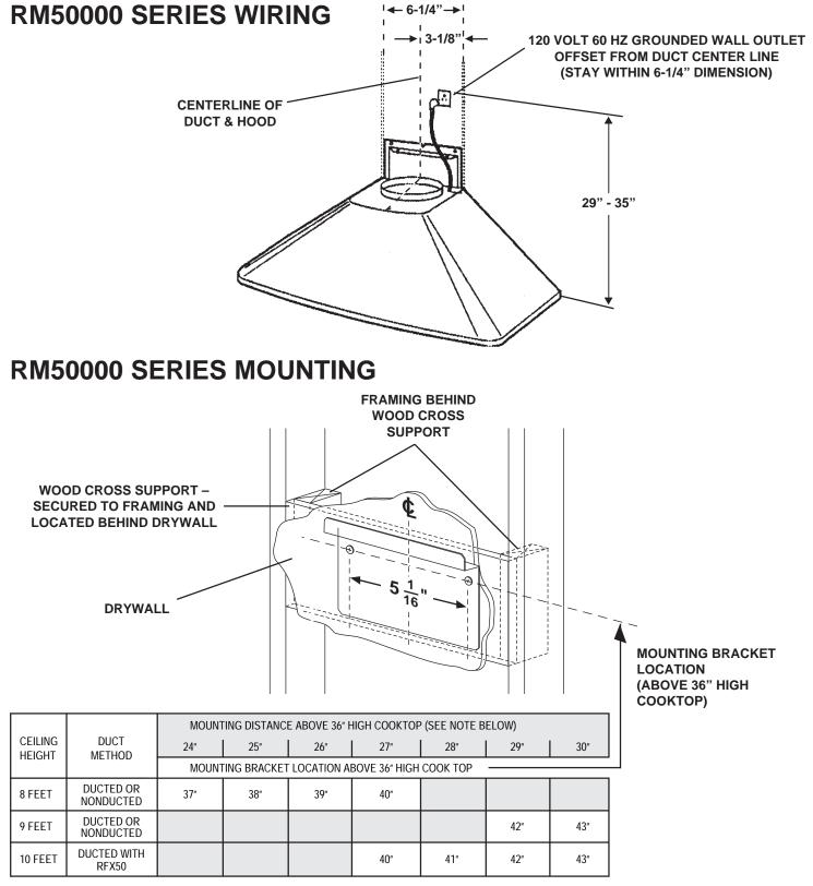
**NOTE:** Minimum hood distance above cooktop must not be less than 24". A maximum of 30" above the cooktop is highly recommended for best capture of cooking impurities. Distances over 30" are at the installer and users' discretion; and if ceiling height and flue length permit.
