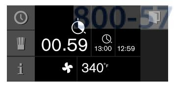
The appliance switches off after expiration of the cooking time. The  $\bigcirc$  pulsates and a signal sounds. It goes off prematurely if you touch the  $\checkmark$  symbol, open the appliance door or set the program selection to  $\bigcirc$ .
