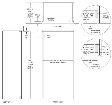
NOTE:  $3^{1}/2^{\circ}$  (89) finished returns and shaded areas will be visible and should be finished to match cabinetry. Shaded line represents profile of unit with  $^{3}/4^{\circ}$  (19) panel.
