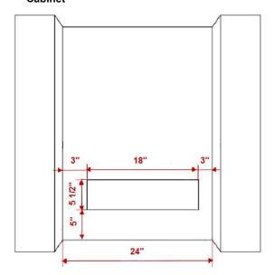
Required minimum air gap clearances: 1/4" sides
