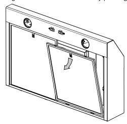
**3** ] Remove both screws holding damper assembly to hood. Remove parts bag included with the hood (captured behind the damper assembly). Remove damper assembly from inside the hood and keep the screws for further use.
