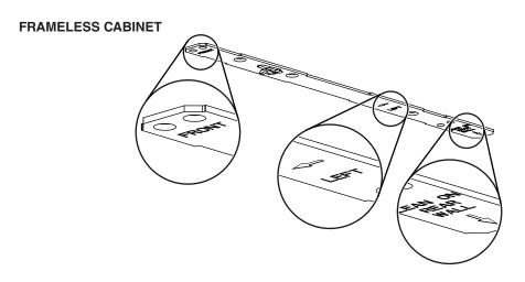
Refer to the marking on brackets to determine the correct installation side and orientation.
