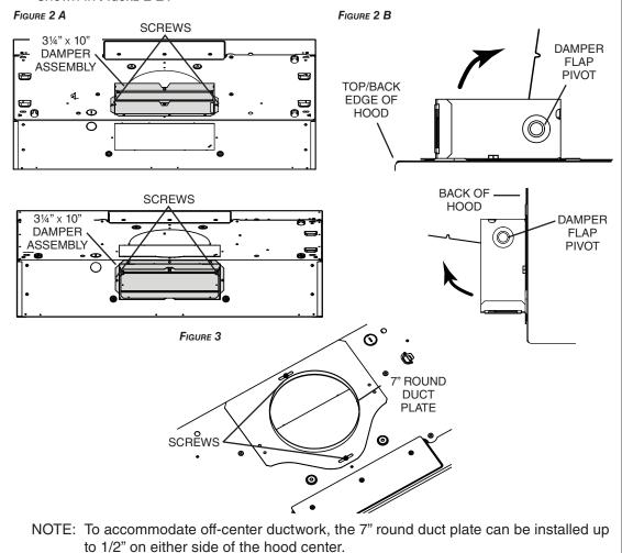
**TIP**: Insert a small length of duct over the 3½" x 10" damper assembly (for rectangular ducting) or 7" round (for round ducting) and seal the joint using aluminum foil duct tape to ease connection with the house ductwork.
