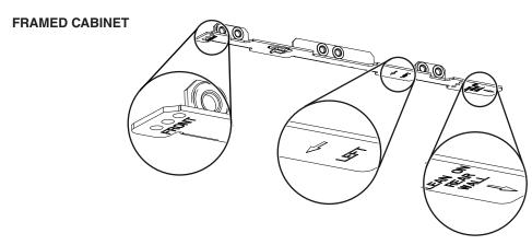
Refer to the marking on the brackets to determine the correct installation side and orientation.
