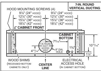
2] Install part-way four (4) ROUND HEAD no. 8 x 5/8" mounting screws into shims/cabinet, according to the proper diagram above. (Mounting screws are included in parts bag, but wood shims and shim mounting screws are not included).
