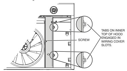
2] Reinstall wiring cover and attach it to the hood using its retaining screw.
