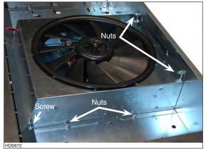
• Remove and set aside the 4 front screws retaining the bent plate to the hood.
