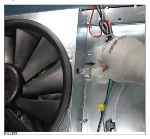
Using a 11/32" socket, remove the 6 nuts retaining the blower chamber to the hood assembly (2 nuts on inner back and 2 other nuts per sides), then use a Phillips no. 2 screwdriver to remove both front corner screws. See picture below for nuts and screws locations. Pull out the blower chamber from the hood assembly and set it aside with its retaining screws and nuts.
