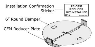
**1.** Remove existing damper and damper clips from blower collar.
