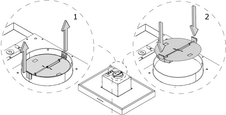
**3.** Firmly press down on CFM reducer clips to secure CFM reducer in place.
