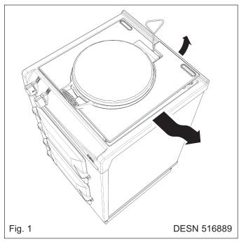
Insert lifting tool in recess at rear of resting plate. Lift up at rear, the slide out carefully from the side, See Fig. 1.
