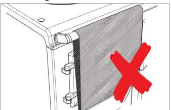
When the oven (s) are on **DO NOT** leave any oven door open for long periods, this will affect the temperature of the oven and may allow controls to become hot.
