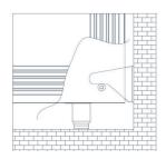
Anti-tip device for CRG3606U
