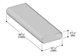
1x AL 400 retractable downdraft with AR 413 722 recirculation blower, AA 413 722 recirculation kit and AD 413 722 flex duct
