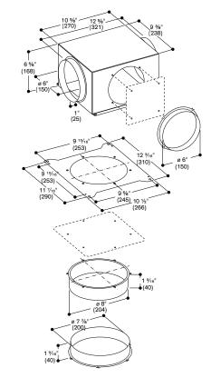
Transition box AD 704 048 for use with AL 400 retractable downdraft
