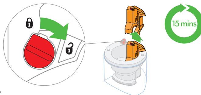
Empty the water tank. To release the water chimney, twist the dial a quarter of a turn. Lift out. Clean thoroughly by immersing in the citric acid solution for 15 minutes. Rinse and wipe over all surfaces. Repeat if necessary. Refit in reverse order, twisting the dial a quarter of a turn to secure.
