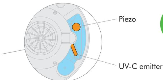
dishwasher. Fill the trough with the recommended acid citric solution until the UV-C emitter and piezo are submerged. Leave for 15 minutes. Drain, rinse and wipe over all surfaces. Repeat if necessary.
