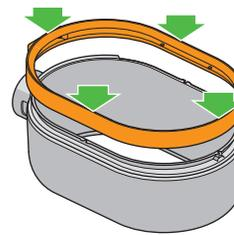
To attach the loop amplifier surround, lie flat and align the surround to the main amplifier. Push firmly until it clicks into place as shown.
