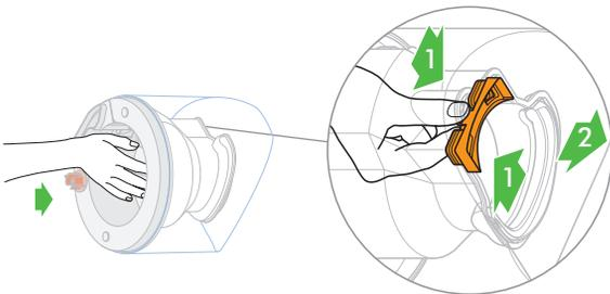
To remove the seal, pinch the securing tabs together and pull out. Clean thoroughly by immersing in the recommended citric acid solution for 15 minutes. Rinse and wipe over all surfaces. Repeat if necessary. To refit, push back in so the tabs click and the fit is secure.
