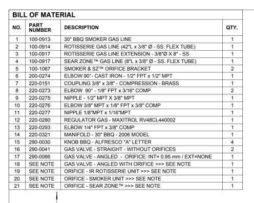
**NOTE:** ORIFICE OR VALVE TO CHANGE ACCORDING TO GAS SUPPLY. (NG OR LP)
