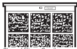
Clogged filter—Greatly reduces cooling, heating and airflow.
