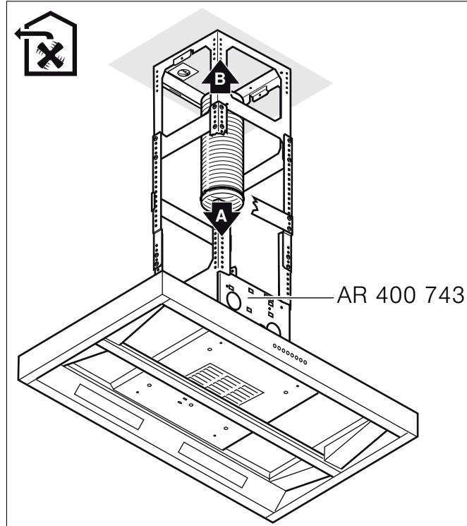
**3 Extraction mode units with external remote fan unit AR 4..:**
