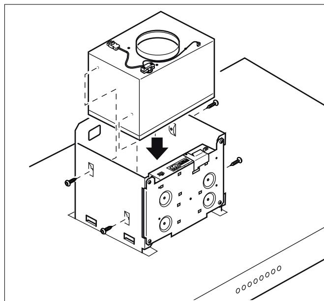
Connect the mains cable and control cable to the control module.
