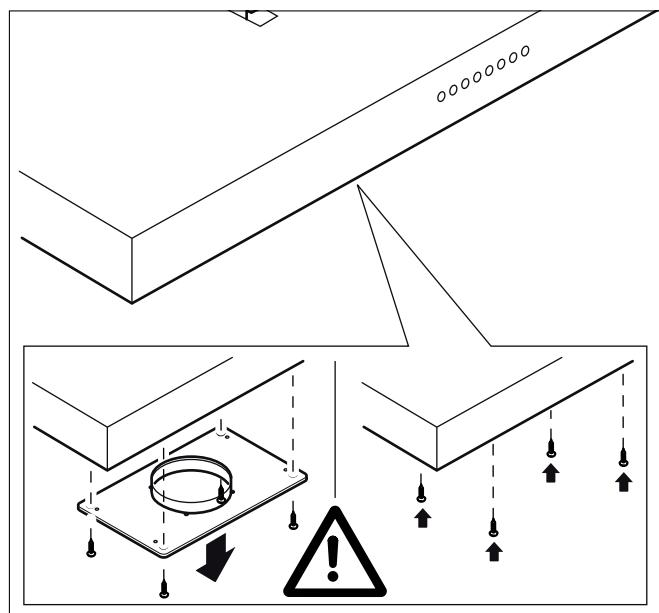
Slide the remote fan unit into the ventilation hood from above. Use four screws to secure it in place.
