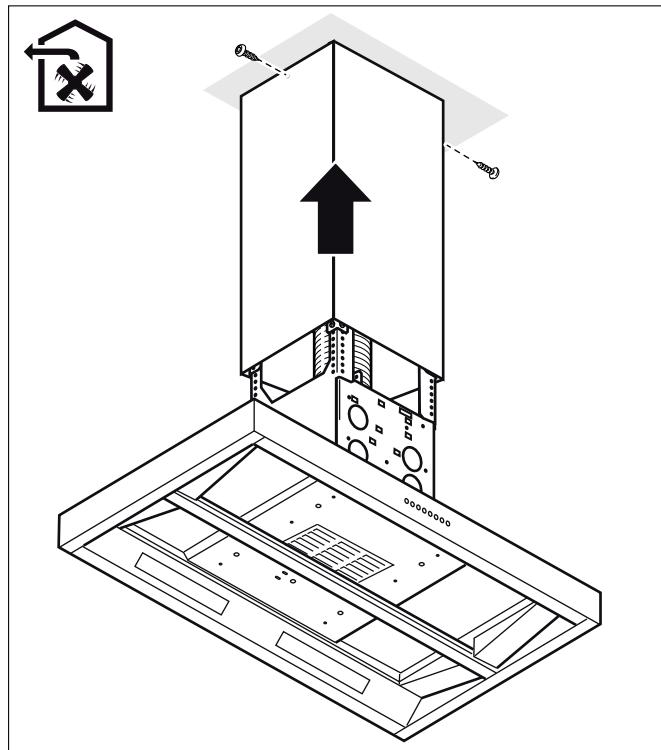
**4** Place both parts of the lower flue duct on the appliance such that they fit together.
