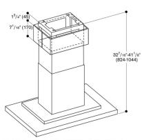
\* Suitable for ceiling heights of 8 ft (2.42 m) to 8.7 ft (2.64 m); Specifications refer to a distance from floor to lower chimney edge of 5.2 ft (1.60 m).
