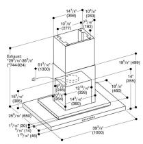
\* Suitable for ceiling heights of 7.7 ft (2.34 m) to 8.3 ft (2.52 m); Specifications refer to a distance from floor to lower chimney edge of 5.2 ft (1.60 m).
