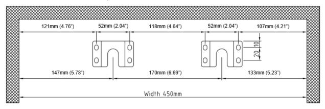
**NOTE:** If the appliance is relocated, the bracket must be removed and installed in the new location.
