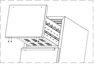
3. Prepare your panel with installation holes and holes for the bottom mounting brackets (20 x 6mm), then secure the mounting brackets to the panel with screws. Be sure to add handle holes to the panel
