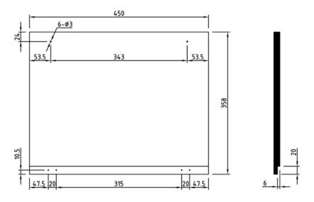
4. Set the panel against the drawer front, and secure it to the bottom of the drawer, with screws. Then, install the handle onto the drawer, through the panel.
