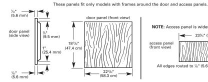
NOTE: Access panel is wider than door panel. 23% (59.2 cm) access panel (front view) All edges routed to 1/2" (5.6 mm) thickness.
