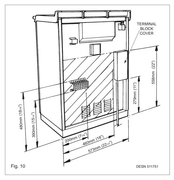
The gas flexiline connector must be fitted in the shaded area indicated in Fig. 10. Take into account that it must be possible to pull the cooker forward sufficiently and that no strain occurs on pipework. Ensure flexiline is not trapped between electrics cover and rear wall. Ensure flexiline is routed within shaded area, and away from the shielded vent.
