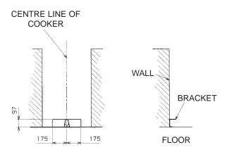
To reduce the risk of tipping, the range must be secured by a properly installed anti-tip bracket supplied with the range. The bracket must be fitted within the shaded area shown in the diagram using  $2 \times 14^n$  fixed in the wall or floor, longer screws may be required depending on the wall or floor covering.
