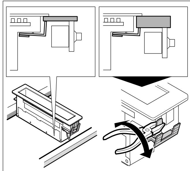
Horizontally insert the appliance in the recess and align it. Tighten the cooktop clamp with the screws in the interior of the appliance.
