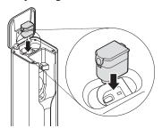
Press the battery down into the compartment.
