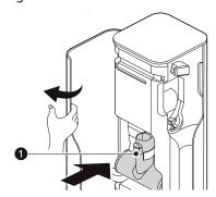
Open the right door and insert the combination tool 2, the crevice tool 3 and the cleaning brush 4 for storage.
