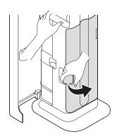
Press ▲ button **1** above the **PUSH** label with one hand. The dust bag is released.
