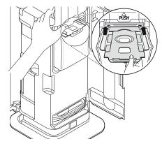
Slide the dust bag in along the rails of the product until it is completely inserted.
