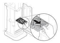
To remove the exhaust filter, hold the bottom of the product and pull the handle end of the filter.
