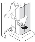
Hold the product with one hand and take out the motor protection filter with the other hand.
