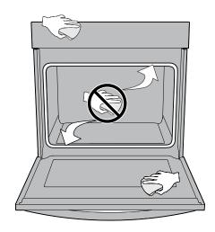
Figure 18: Clean around the oven door gasket
