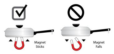
Figure 4: Magnet test
