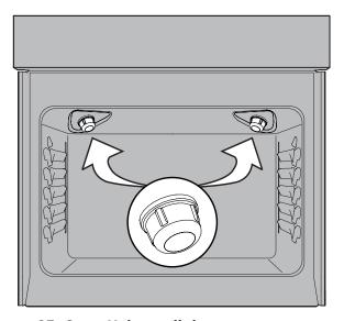
Figure 23: Oven Halogen light
