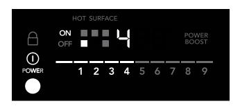
5. When cooking is complete, turn the induction cooking zone off by pressing its **ON-OFF** key or the **Power** key before removing the cookware. If all of the zones are off, the cooktop will automatically power off in 30 seconds.
