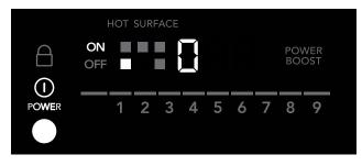
4. Press **4** on the power level selection bar. The power level indicator will show 4.
