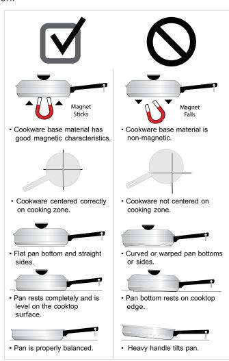
Figure 5: Pan sensing conditions
