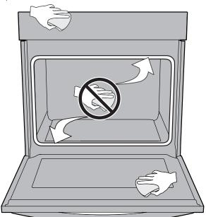
Figure 20: Clean around the oven door gasket
