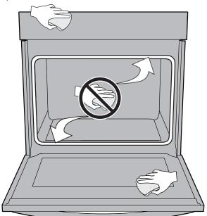
Figure 15: Clean around the oven door gasket
