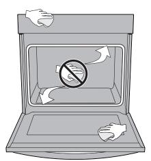
Figure 17: Clean around the oven door gasket
