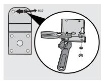
6. Unscrew the left adjustable leveling foot and loosen the screw.
