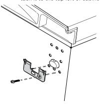
Insert the hinge into the positioning guide. Move the door up and insert the hinge pin. Attach the hinge onto the cabinet with screws
