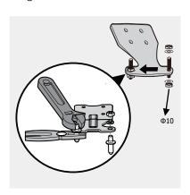
With a flat head screwdriver, gently pry upward on hinge pin bearing to remove from door. Reinstall on the opposite side of the door.
