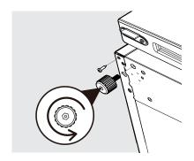
Attach the bottom hinge (A) with 4 screws (B) and the adjustable leveling foot (C) on the left side of the cabinet.
