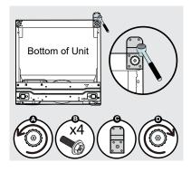
Unscrew the door stopper on the right side with a Phillips screwdriver and pry off the stopper with a flathead screwdriver. Then screw it on the left side.
