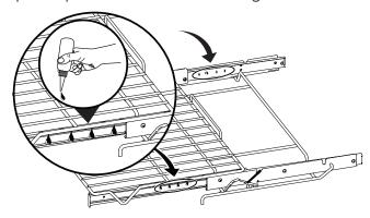
4. Extend and return the glide rack several times along the tracks to distribute the lubrication.
