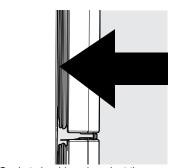
Gasket should seal against the cabinet all the way around including top and bottom
