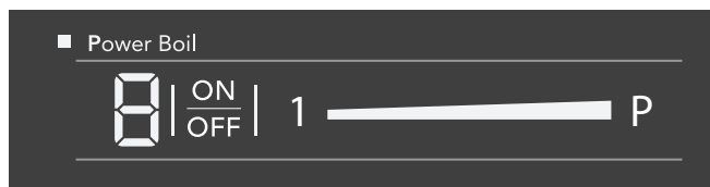
Figure 12: Induction cooking zone control
