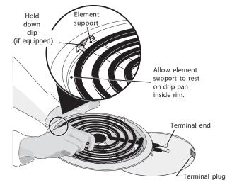
Figure 13: Removing coil and drip bowl
