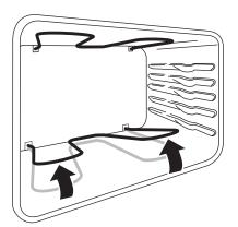
Figure 14: Lift bake element
