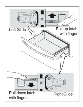
Figure 21: Parts of storage drawer
