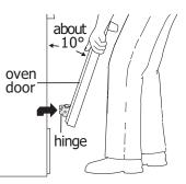
Figure 18: Holding door for removal
